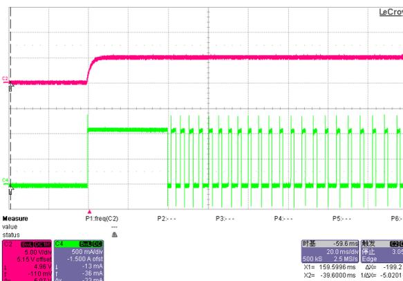
Device Enabled into short-Circuit
