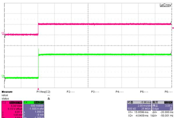
Device Enabled into short-Circuit
