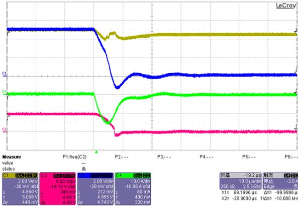
Input Voltage from 5V into 0V
